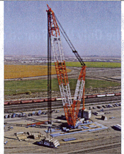
BIG MUSCLES Lampson's latest heavy lifter has been updated with hydraulically operated hoists.
