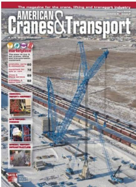
The massive crane, with a rated capacity of 2,600 tons, will be loaded onto three barges in the Port of Pasco, WA. The barges, with a capacity of 800 to 1,000 tons each, will move the crane down the Columbia River to Vancouver, WA, according to Brian Pepin-Donat, director of contracts and international business for Lampson.
